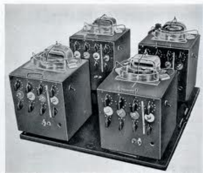
Fig. 1.—The homeostat, with its four units, each one of which reacts on all the others.
