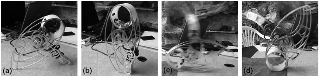
Fig. 5 The robot SEMNI exhibits two revolute joints, namely a hip joint and a knee joint, which are both controlled by the presented cognitive sensorimotor loop (CSL). The robot always defies gravity. When placed as shown in (a), the robot targets an upright position (b). Starting from the position shown in (c), the robot increasingly vigorously rocks back and forth until it almost comes to rest in headstand (d). After a second the robot rolls onto his leg and again ends up in a fully vertical headstand, as shown in panel (f) of Figure 6.
